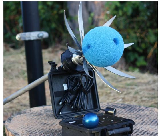
The SmartBall tool rolls along with the flow of pipeline, identifying leaks and gas pockets while the line remains in service, minimizing disruption.
