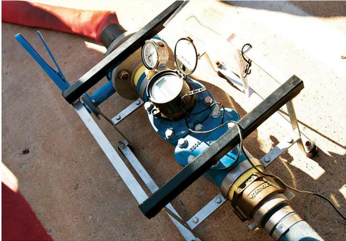
The portable OMNI Verification (V<sup>2</sup>) portable test meter is placed in-line to check the accuracy and performance of large, commercial meters without interrupting service.
